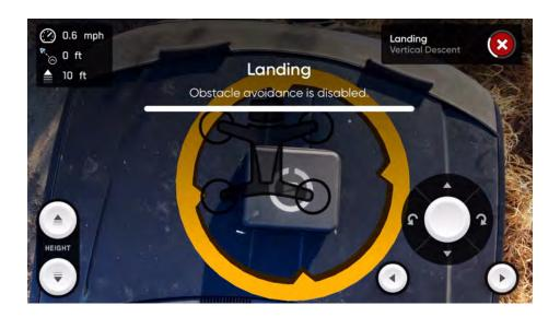
Piloting or nudging the vehicle during a case landing will cancel the case landing and continue with a normal landing.
