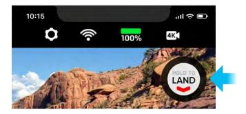
Skydio 2 will descend until it is 3m (10 ft) above the surface below it. Once Skydio 2 is less than 3m from the surface the LEDs on Skydio 2 will turn yellow and all obstacle avoidance will be disabled for the remainder of the landing. Users will be notified of this change on screen if flying with the Skydio 2 app.
